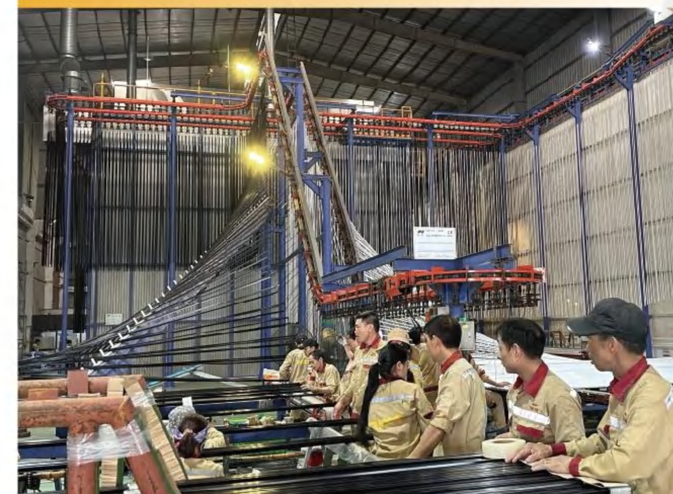
Automatic Powder Coating Line
