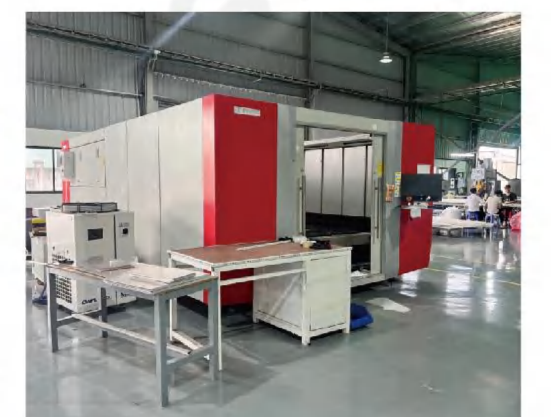
Sheet Metal Laser Cutting Line
